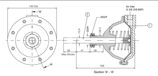
This range of pneumatically operated brakes uses dry and filtered compressed air at pressures up ot 7 bar. Pneumatic brakes require a control valve which may be operated either manually, or by pneumatic or electrical signal.
